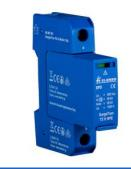
TT systems, providing optimum protection against temporary overvoltages (TOV) caused even by faults in medium voltage. It is providing protection against surge currents up to 65 kA (8/20  $\mu$ s). The residual voltage is less than 1,5kV (@ 20 kA) providing complete protection to equipment of all categories of insulation level (category IV up to category I) according to IEC 60364-4-44\*.
