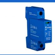
TT systems, providing optimum protection against temporary overvoltages (TOV) caused even by faults in medium voltage. It is providing protection against surge currents up to 65 kA (8/20  $\mu$ s). The residual voltage is less than 1,5kV (@ 20 kA) providing complete protection to equipment of all categories of insulation level (category IV up to category I) according to IEC 60364-4-44\*.
