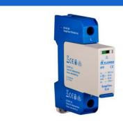
systems, providing optimum protection against temporary overvoltages (TOV) caused even by faults in medium voltage. It is providing protection against surge currents up to 50 kA (8/20  $\mu$ s) per pole, 200 kA (8/20  $\mu$ s) per 4 poles. The residual voltage is less than 1,75kV (@ 20 kA) providing complete protection to equipment of categories of insulation level IV up to II, according to IEC 60364-4-44.
