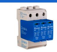
to electrical systems of insulation level, category III and category IV according to IEC 60364-4-44. It is suitable for direct installation exactly at the input terminals of the inverter just after the entrance of the DC current arriving from the photovoltaic panels. Its main advantage is that no back up fuse is required for up to 30 kADC expected short circuit current.
