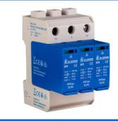
electrical systems of insulation level, category III and category IV according to IEC 60364-4-44. It is suitable for direct installation exactly at the input terminals of the inverter just after the entrance of the DC current arriving from the photovoltaic panels. Its main advantage is that no back up fuse is required for up to 11 kADC expected short circuit current.
