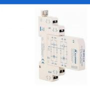
installed in switchboards and control panels with limited space and where a numerous of incoming and outcoming cables are connected, such as interfaces RS 485 and RS 422. Quick and easy installation by clipping on DIN rail. It is consisted of a plug-in protection module and a base. The signal pass through the base in order to operate uninterruptible even with the module removed. The plug-in protection module can be replaced in no time with no need to cut-off the signal.
