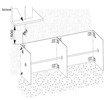
Installation of earth electrode type "E"™. Burried in ground.
