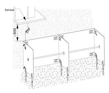
Installation of earth electrode type "E"™. Embedded in concrete.
