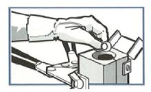
Close mould properly with the handle clamp to prevent molten metal leaks.
