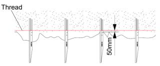
For uneven surfaces, with a variation up to 100 mm, install the first fastener at the higher point of the trench's bottom. Drive the first fastener into the soil, up to the notch. Use a thread in order to drive the tape receptacle of the other fasteners into the same level with the tape receptacle of the first fastener.
